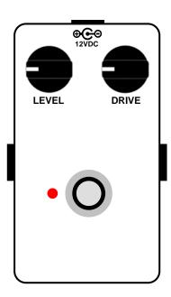
This pedal is designed to operate from 12DVC. The "9VDC Mod" can be performed by bridging the two points shown.
